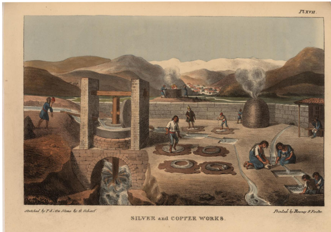
FIGURE 2. A depiction of the patio process using mercury amalgamation at a historic silver refinery in Chile. (Sketch by Peter Schmidtmeier, 1824. Courtesy of the John Carter Brown Library, Brown University.)
