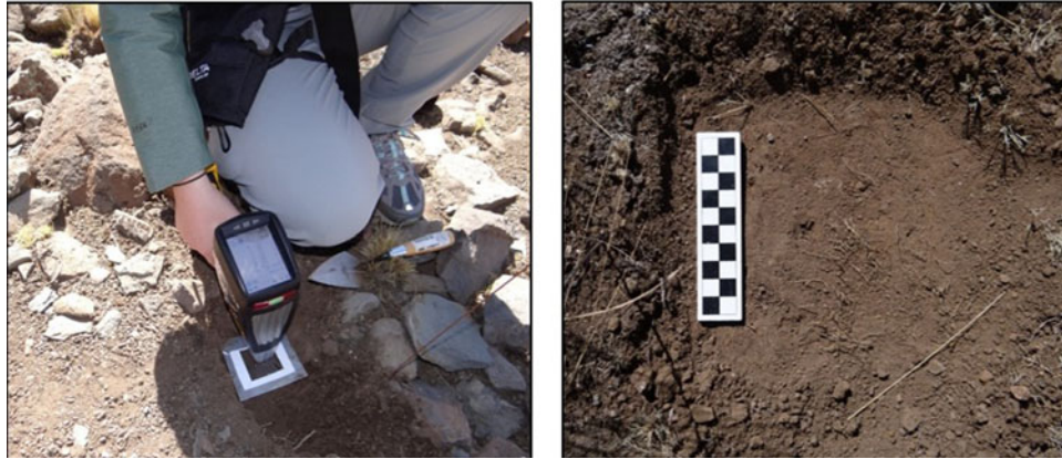
FIGURE 6. (Left): the pXRF instrument was pressed to the soil to take readings, and a polypropylene protector film was placed over the sample area to keep the instrument window clean and protected from damage; (Right): photographs were taken of sample locations, which were cleared of brush and the first 3–5 cm of topsoil before analysis.
